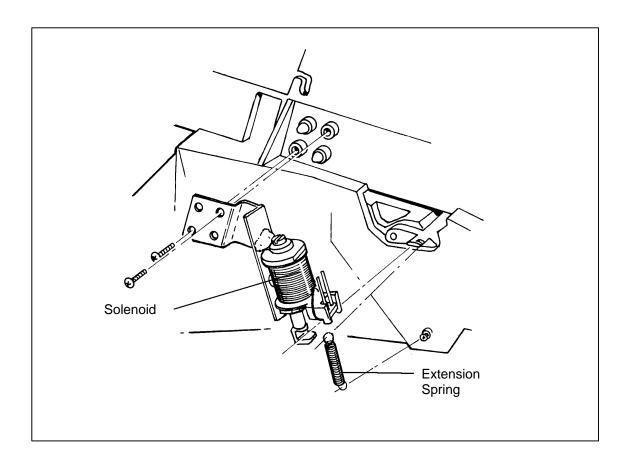
Figure 5-14 Shutter Solenoid Assembly
